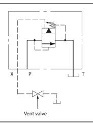
Hydraulic Remote Control Remote adjustment of pressure setting can be made by a pilot relief valve, substituted for the vent valve in the diagram. Suitable pilot relief valves are described in catalogs 411 (type C-175 valves) and 409 (type CGR-02 valves). Control Data for CG5V Valves Vent Function
