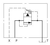
Sequence valve, manually adjusted, CG2V-\*\*\*- 1-1\* model ▲
