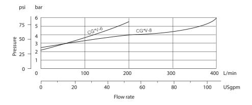
Control Data for CG2V Valves Manual adjustment of pressure setting described in "Installation Dimensions".
