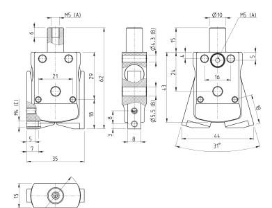
A = port connection B = mounting holes C = mounting thread
