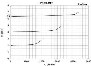
Pr = Regulated pressure (bar) Q = Flow (Nl/min) Pa = Inlet pressure (bar)
