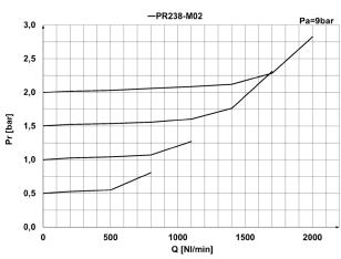
Pr = Regulated pressure (bar) Q = Flow (Nl/min) Pa = Inlet pressure (bar) EXHAUST FLOW
