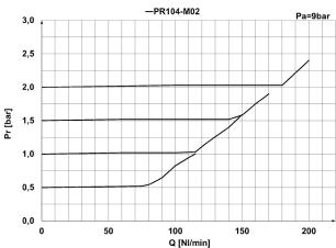
Pr = Regulated pressure (bar) Q = Flow (Nl/min) Pa = Inlet pressure (bar)
