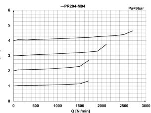
Pr = Regulated pressure (bar) Q = Flow (Nl/min) Pa = Inlet pressure (bar) EXHAUST FLOW
