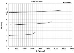
Pr = Regulated pressure (bar) Q = Flow (Nl/min) Pa = Inlet pressure (bar) EXHAUST FLOW
