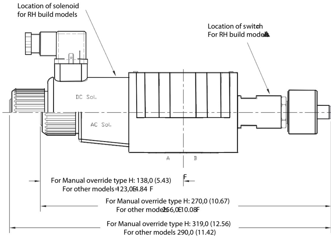
▲ For LH models ("L" in model code location 4) solenoid and switch locations are reversed
